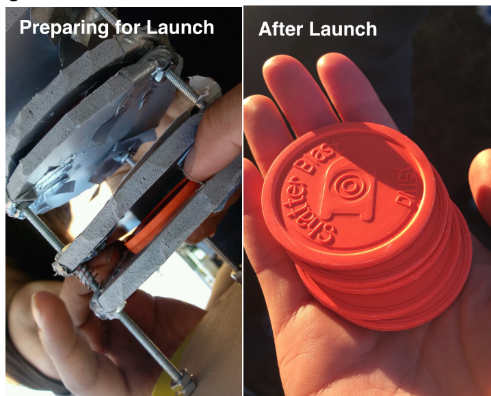
Figure 5 displays an independent fragile material incorporated into a compartment within the payload inner rack prior to launch (left) as well as the mint condition of the fragile material post launch (right).
