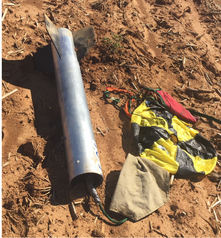
Figure 9 shows the booster section of launch vehicle after landing, it sustained no damage during or after flight.
