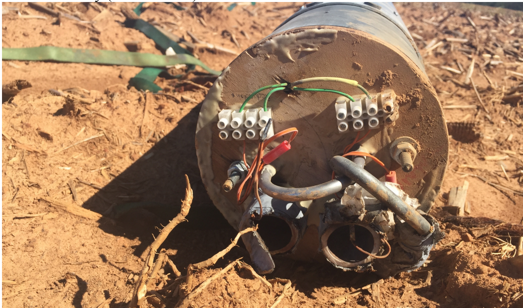
Figure 8 displays the condition in which the avionics bay was found after landing. All wires remained intact and connected. The ejection charge canisters or the avionics bay did not substantiated any damage. Both ejection canisters displayed clear indications that the main and redundant charged occurred during launch.
