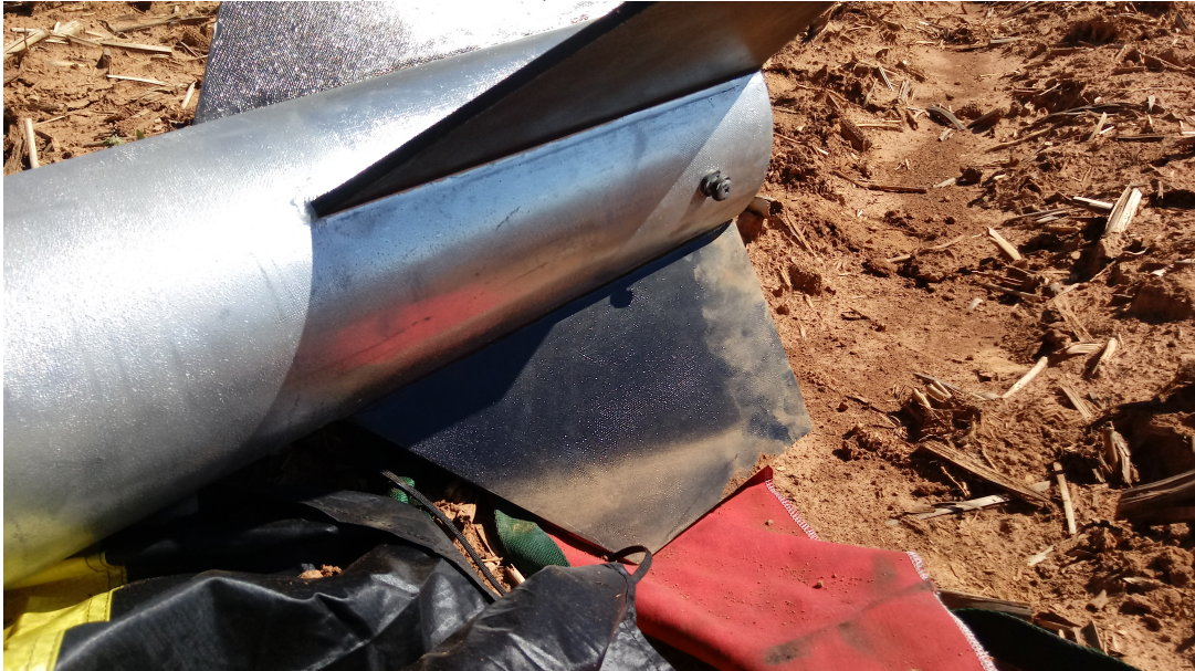
Figure 7 shows the condition in which the fins were found after landing. Fins did not show any evidence of cracking or splintering and all connections were intact.
