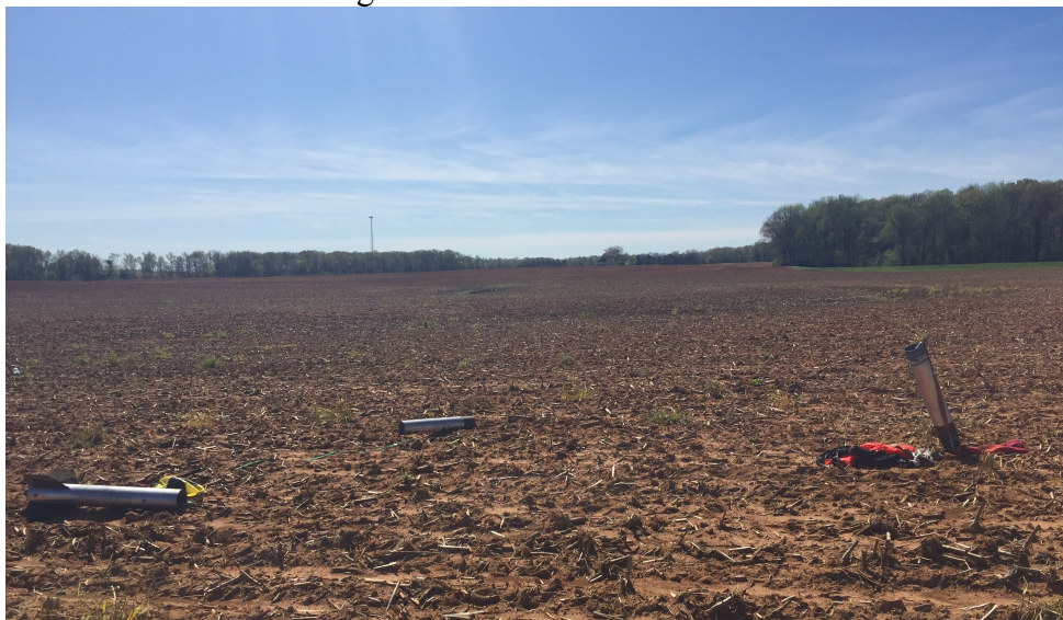
Figure 6 shows a side view of the launch vehicle after landing. The nose cone pierced the ground but sustained no damaged. All connections between the sections of the rocket remained secured and the vehicle showed no signs of damage.
