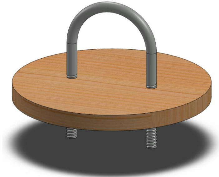
Figure 9 shows the bulkhead that will be used in the booster section and payload bay.
