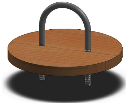
Figure 21 shows the 0.3125 in U-bolt that will be secured onto a 0.5 in thick 5-ply wood bulkhead to be attached to the 6 in diameter airframe
