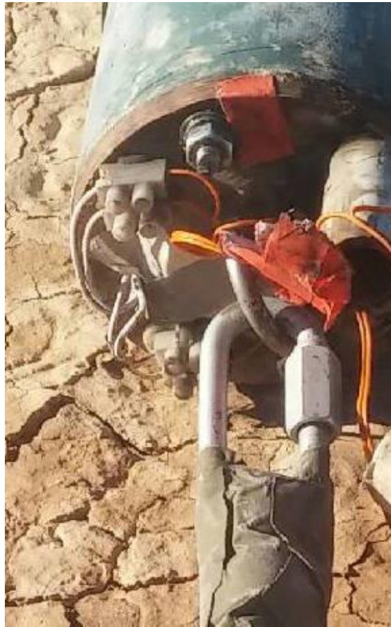
Figure 20 shows the 0.25 in quicklink attached to the U-bolt secured onto the bulkhead of the avionics bay.
