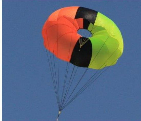
Figure 19 shows the 120 in diameter toroidal ripstop nylon main parachute that will be used in Project Aegis.
