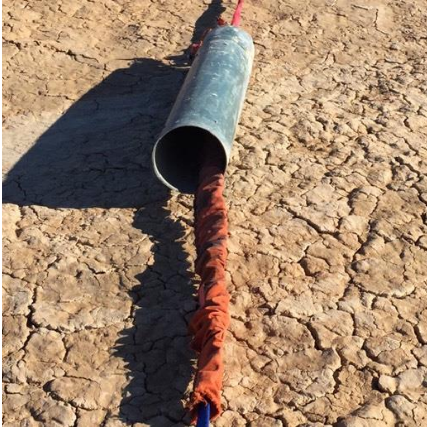
Figure 23 shows the nomex sleeves that protect shock cords from the high temperatures of the ejection gases.
