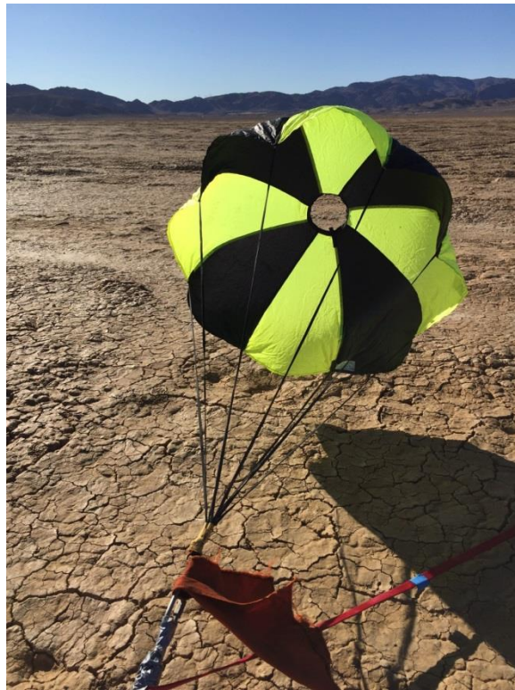
Figure 18 shows the 24 in diameter elliptical ripstop nylon drogue parachute that will be used in Project Aegis.
