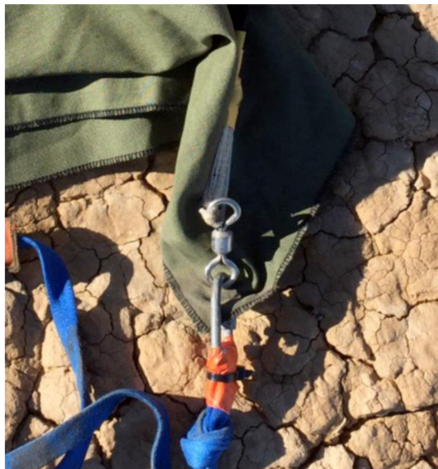
Figure 22 shows the interfaces of the shroud lines, eyeswivel, quicklink and shock cord.
