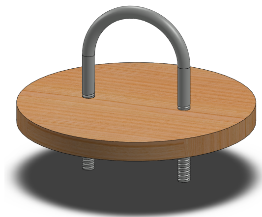
Figure 12: Bulk Plate with U-Bolt (Isometric View)
