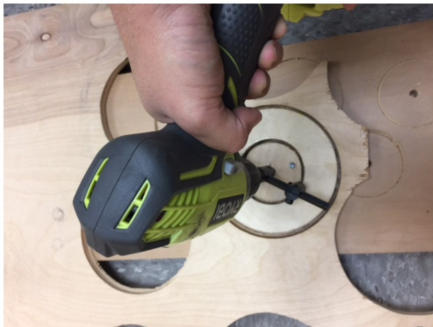
Figure 6 shows how the 0.50" centering rings were constructed out of 5-ply birch wood.
