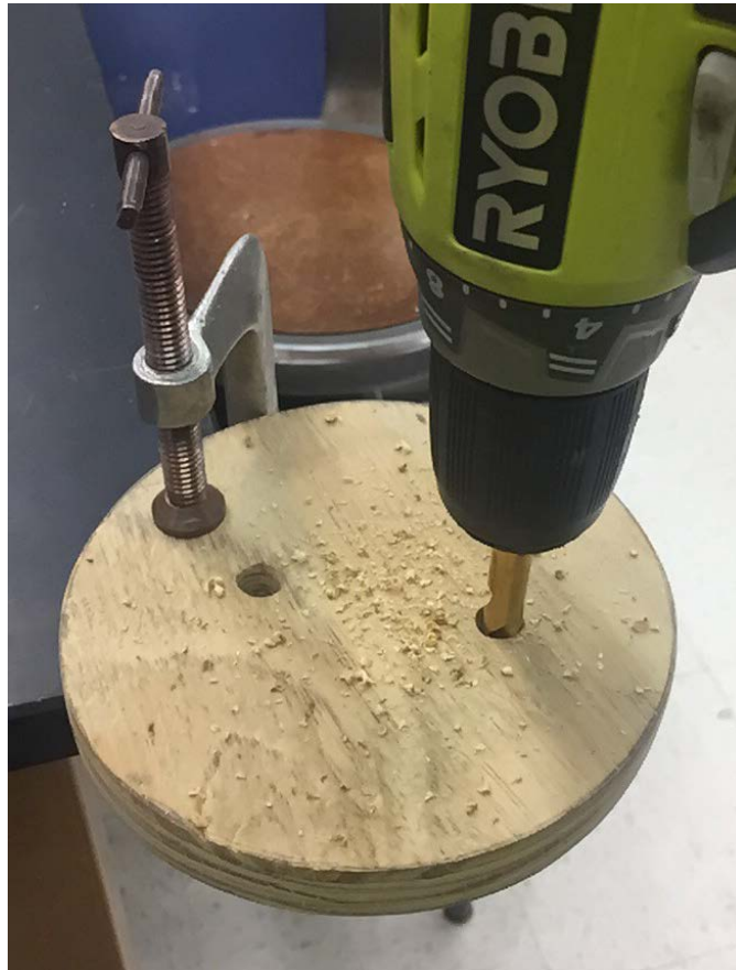
Figure 9 shows how the bulkheads were drilled in preparation for bulkhead installation.
