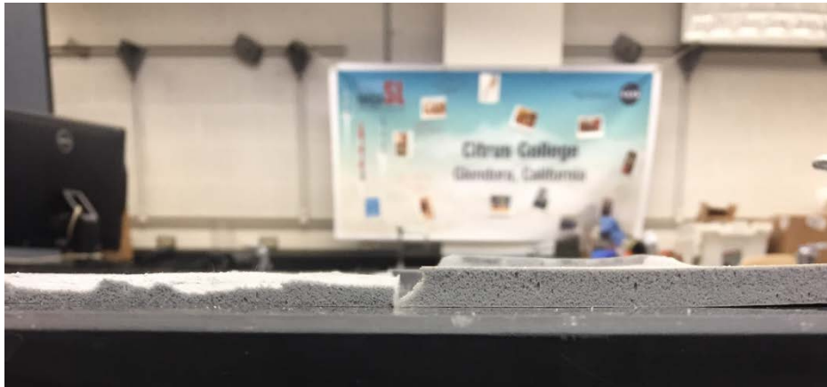
Figure 64 shows the thinned layer of silicone rubber used in the payload.
