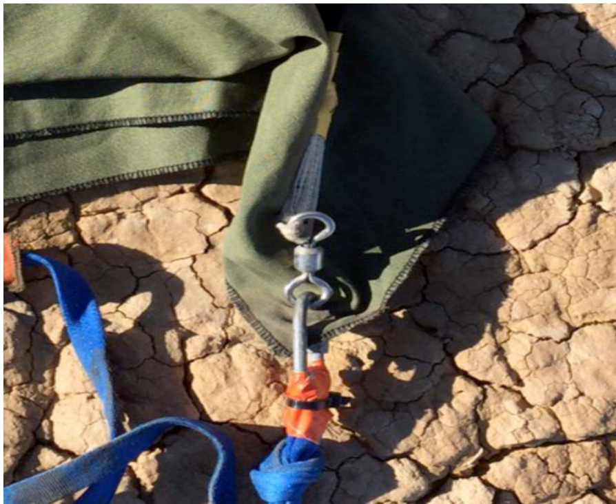
Figure 22 shows the interface between the shroud lines, eyeswivel, quicklink and shock cord.
