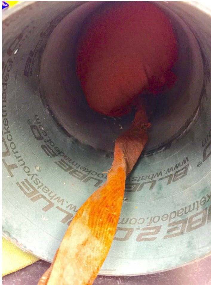
Figure 25 shows the main parachute wrapped in the 24" nomex blanket.
