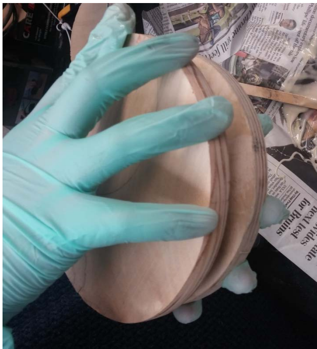
Figure 12 displays the two avionics bulkheads being epoxied together.
