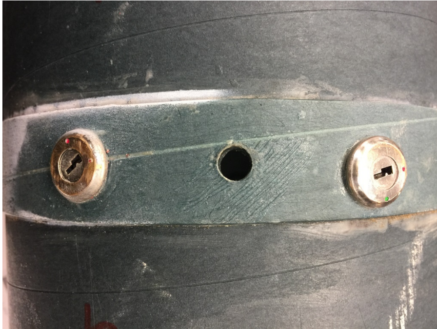
Figure 44 shows the two key switches on the avionics switch panel.
