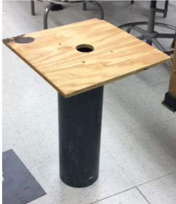
Figure 14 displays the fibreglassed Blue Tube set up prior to adding mass for testing.
