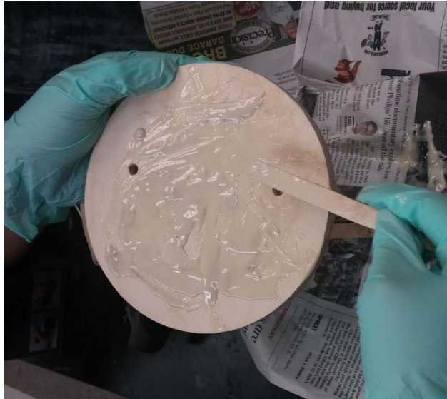
Figure 11 shows the epoxy being applied to the top bulkhead of the avionic bay.
