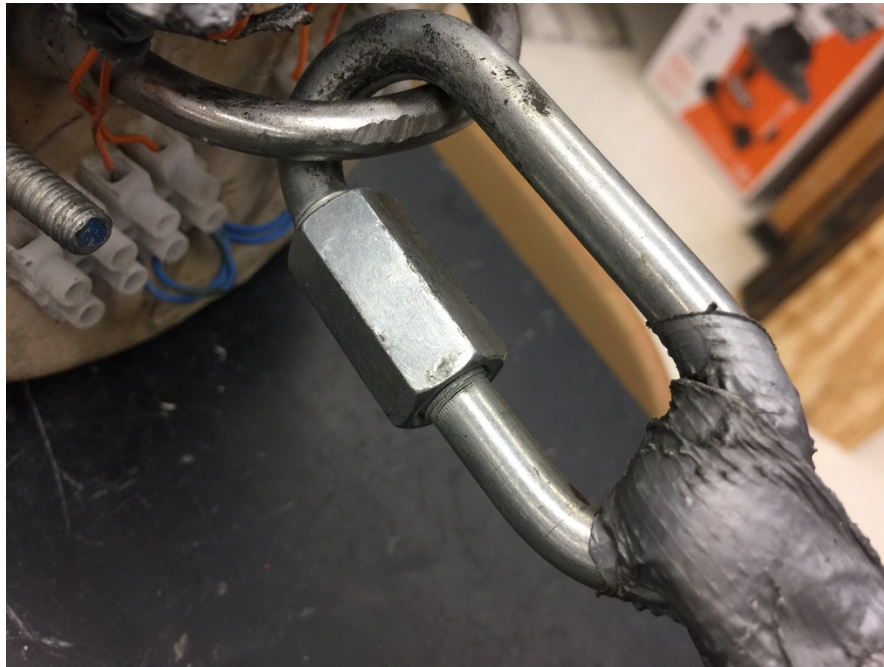
Figure 23 shows the 0.3125" quicklink attached to the 0.3125" u-bolt secured into the bulkhead of the avionics bay.
