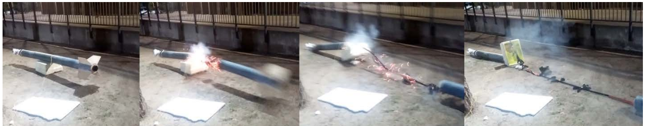
Figure 90: Displays the complete ground ejection test of the drogue parachute.
