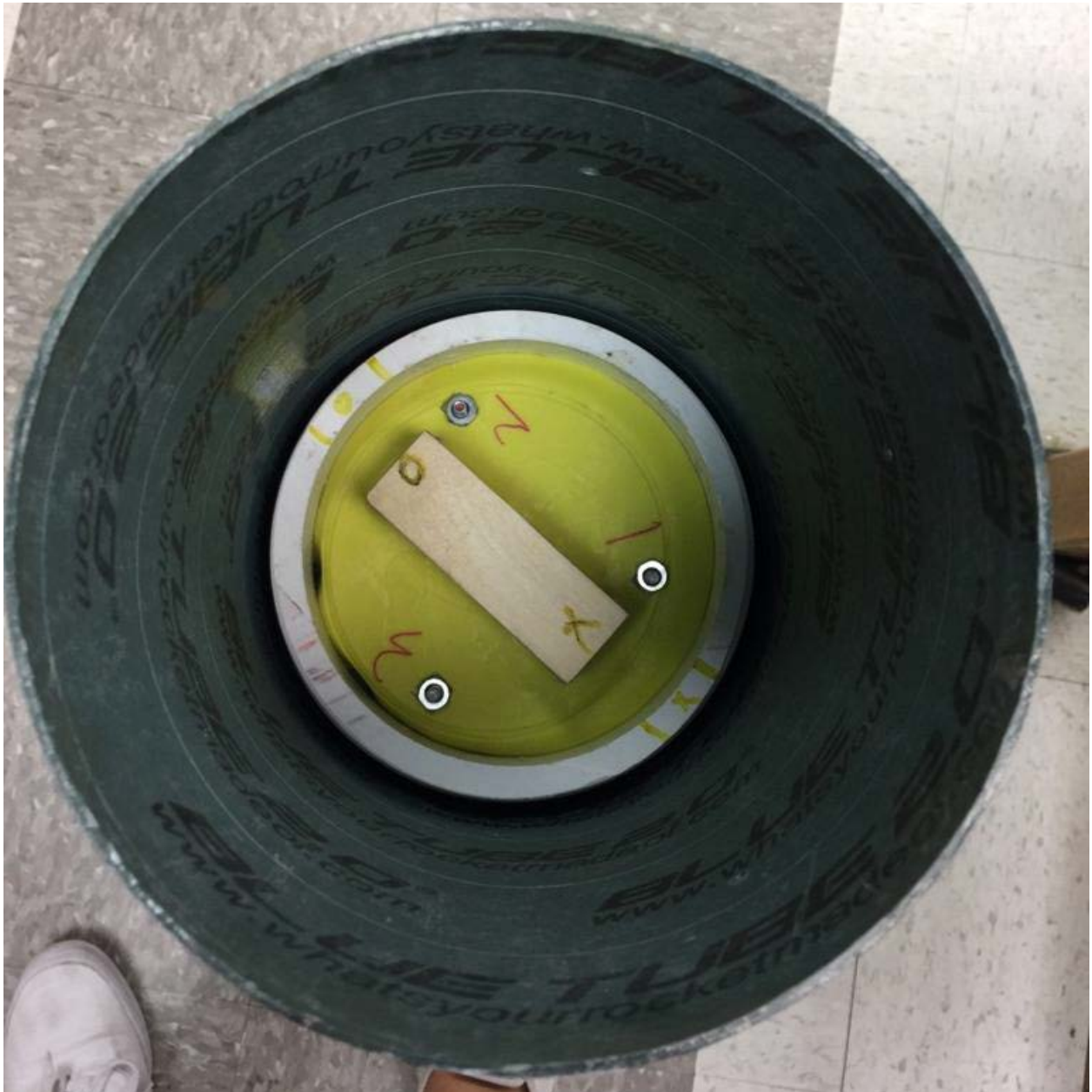
Figure 76 shows the payload body inside the forward section as the foam mold is being made
