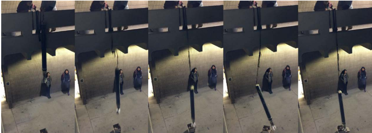
Figure 29 shows the second drop test with the elastic cord attached to the shock cord knots.
