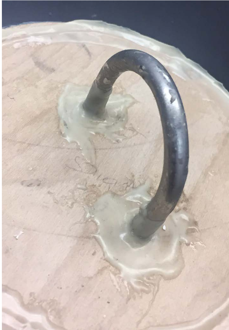
Figure 10 displays the U-bolt secured onto the bulkhead using epoxy.
