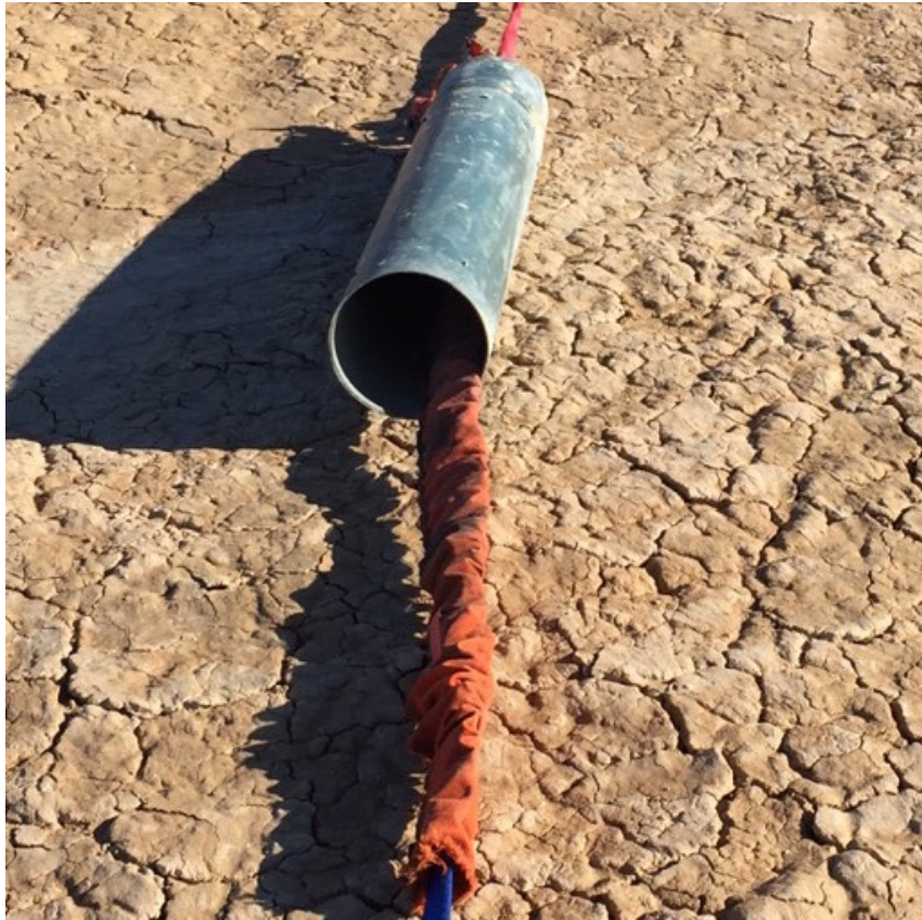
Figure 26 shows the nomex sleeves that protect the shock cords.
