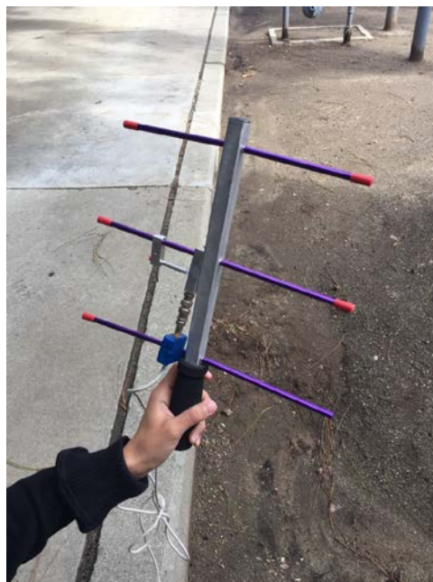
Figure 57 shows the Yagi Antenna that receives the frequency of the transmitter.
