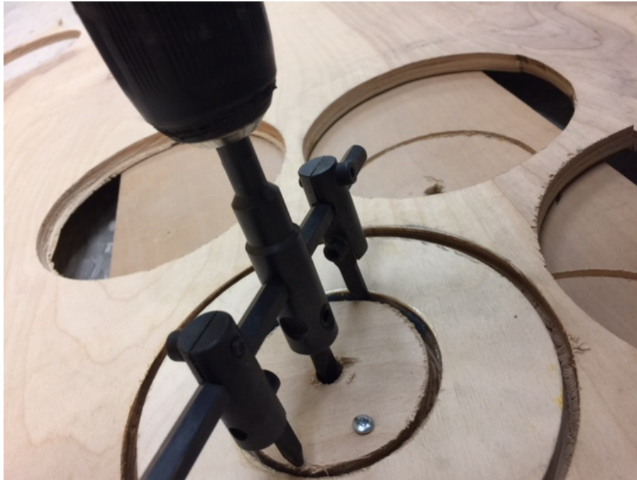
Figure 5 shows the centering rings being cut using an adjustable circle cutter.
