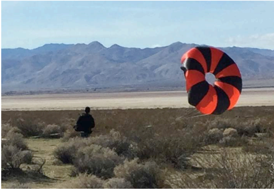
Figure 21 shows the 120" diameter toroidal ripstop nylon main parachute used in Project Aegis.
