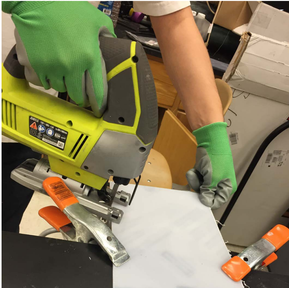
Figure 78 shows how the base of the outer shell was cut.
