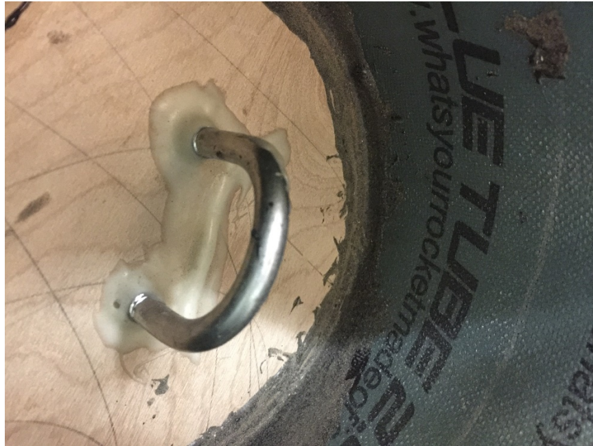
Figure 24 shows the 0.3125" u-bolt that will be secured into a 0.50" thick 5-ply wood bulkhead to be attached to the 6" diameter airframe.
