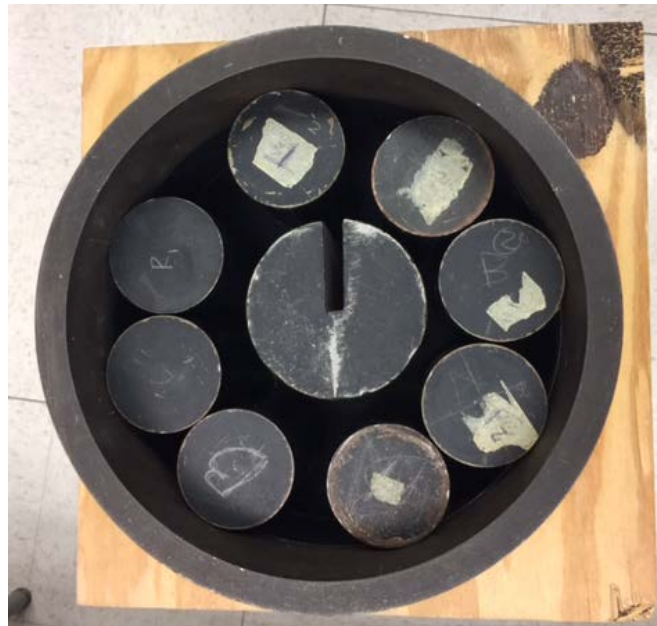
Figure 15 shows how the weights were arranged in the bottom layer to keep the force evenly distributed on the Blue Tube.
