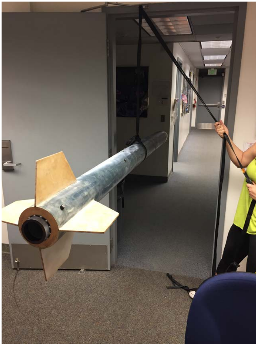
Figure 19 shows the configuration for the completed center of gravity test.
