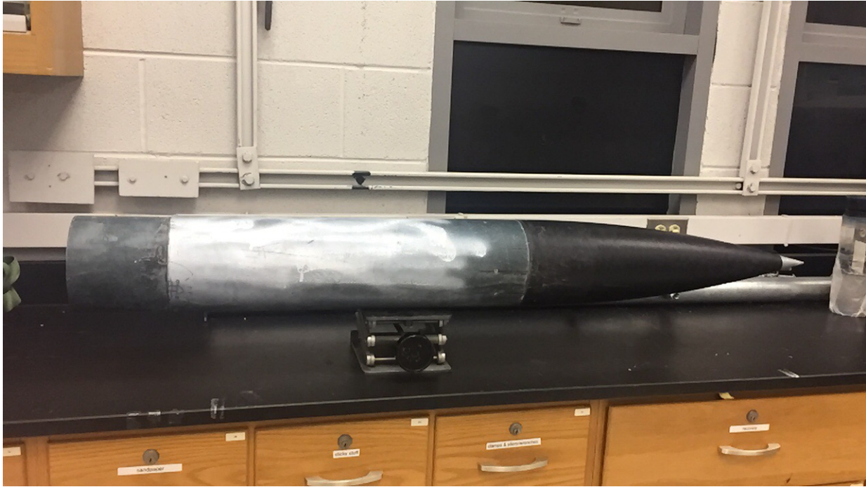
Figure 4 shows the fully assembled forward section of the launch vehicle.
