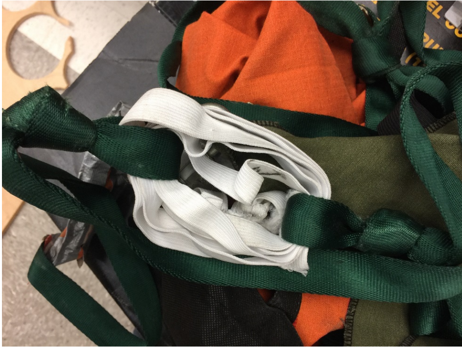
Figure 27 shows the attachment of the elastic cord to the two knots tied on the shock cord.
