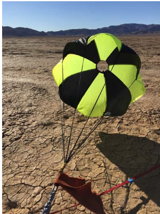
Figure 20 shows the 24” diameter elliptical ripstop nylon drogue parachute used in Project Aegis.
