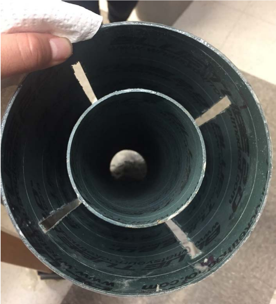
Figure 8 displays the installation method for the fins.
