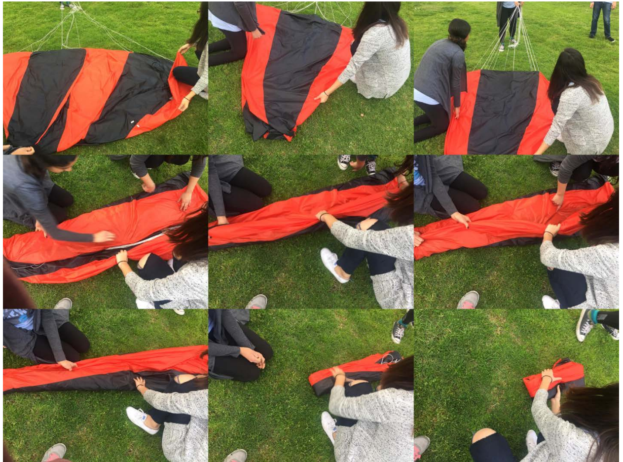
Figure 88 shows the process used to fold the parachute before the parachute run test.
