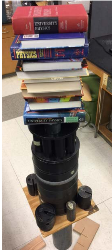
Figure 17 displays the final set up of the compression test with a total mass of 409 lbs.
