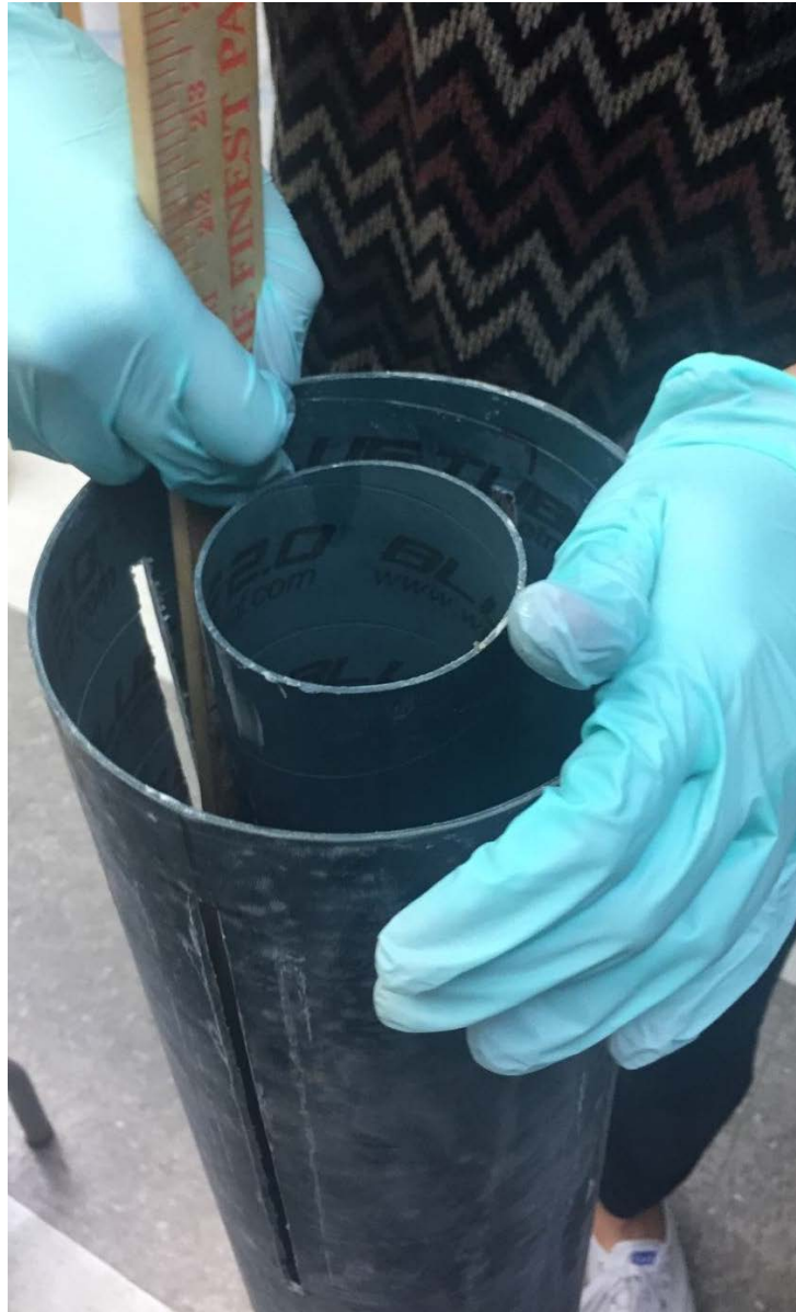
Figure 7 shows the method used to fillet the inner and outer diameters of the centering rings to adhere them to the motor mount and airframe.
